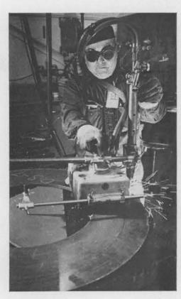
GEORGE TORRES burns a circle out of sheet metal using a semi-automatic positioning device. The machine automatically cuts any size circle to within 1/32-inch accuracy.
